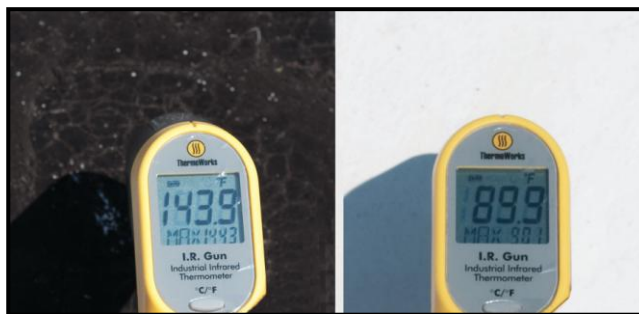
Figure 1: Dark vs. Cool Roof Surface Temperatures
